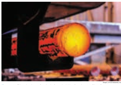
Figure 29-28. This steel coming out of a preheating furnace is a bright yellow color at 2400 F (1320 C).
