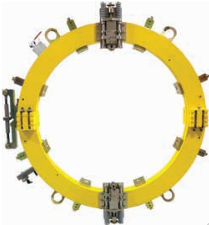
Figure 25-13. A hydraulic lathe tool is attached to the pipe to be cut. A cutting and optional beveling tool are driven around the pipe to prepare the pipe for welding.
