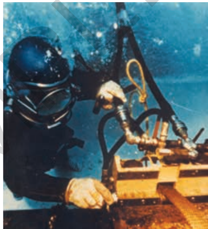
Figure 25-12. A hydraulic milling machine. A—This machine cuts and bevels the end of a pipe in preparation for welding. B—Underwater cutter in use.
