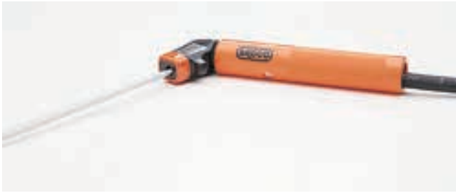
Figure 25-3. An underwater SMAW electrode holder. The holder is well-insulated, with no bare metal areas.
