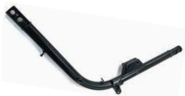
Figure 18-5. Double cradle frame. A—Note how triangles are often formed at junctions of cradle frame tubes. B—Down tube removed from frame. Note the holes that allow the down tube to be bolted and unbolted from the frame.
