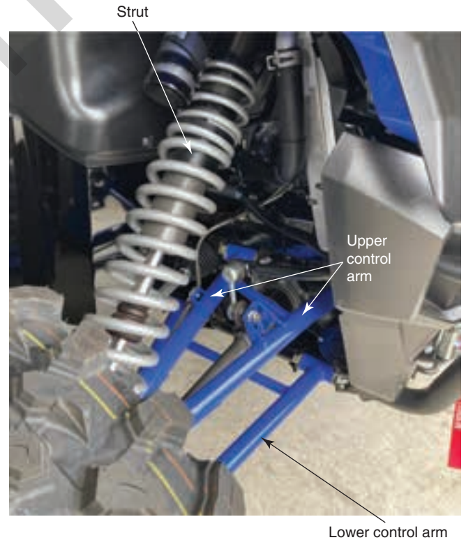
Figure 18-13. ATV and UTV front suspension systems are similar to automotive front suspension systems. Note the upper and lower control arms and strut.
