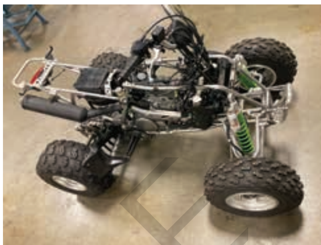
Figure 18-3. An ATV frame serves the same function as a motorcycle frame.
