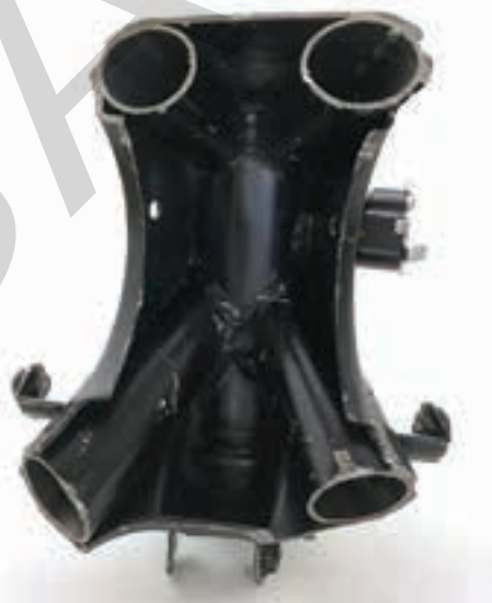
Figure 18-2. Frame cross sections. A—Cross section of a steel frame made up largely of round tubing. B—Cross section of an aluminum frame.
