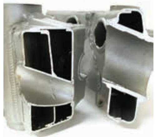
Figure 18-2. Frame cross sections. A—Cross section of a steel frame made up largely of round tubing. B—Cross section of an aluminum frame.
