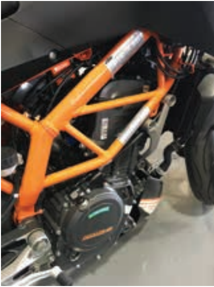
Figure 18-1. The primary function of the frame is to provide a non-flexing platform for the engine, suspension, and wheels.
