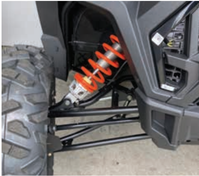
Figure 18-38. Caster, camber, toe, and thrust angles must be measured and compared to specification when performing a four-wheel alignment on an ATV or UTV.
