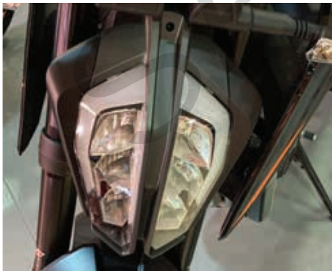
Figure 12-6. An LED headlight equipped on a motorcycle.
