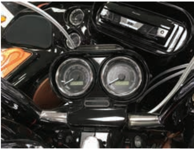
Figure 12-21. An analog speedometer and tachometer.
