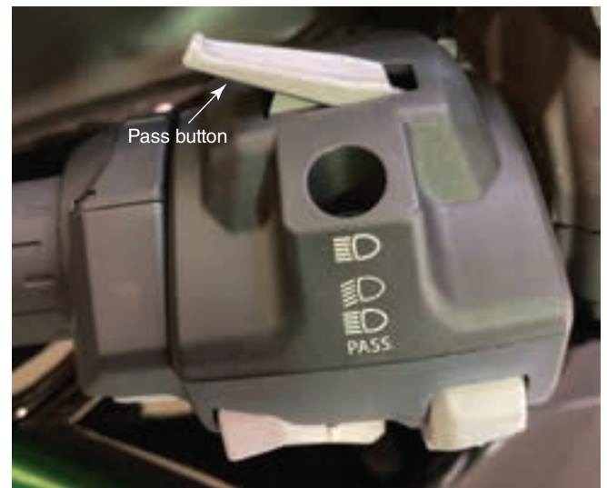
Figure 12-9. The pass button turns on the high beam when pressed and returns to low beam when released.
