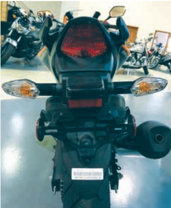
Figure 12-10. Typical taillight, brake light, and license lamp assembly.
