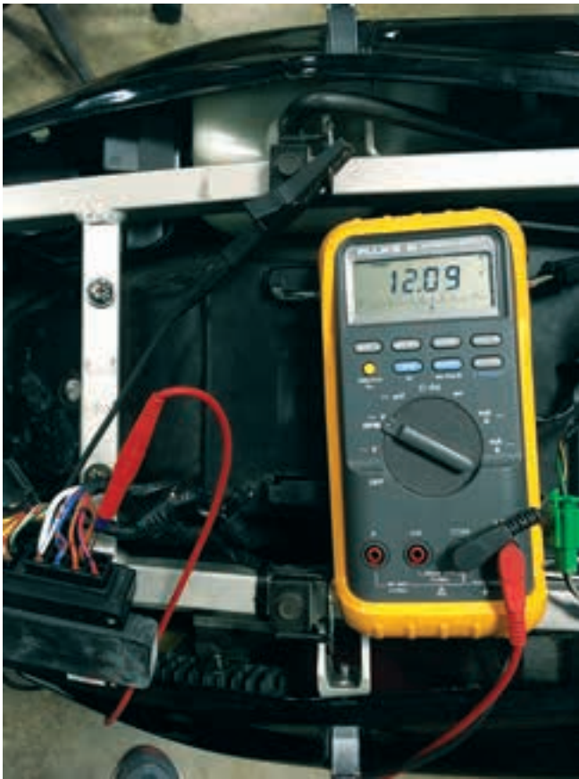
Figure 12-16. A multimeter can be used to check for voltage at the headlight or other plug connections.
