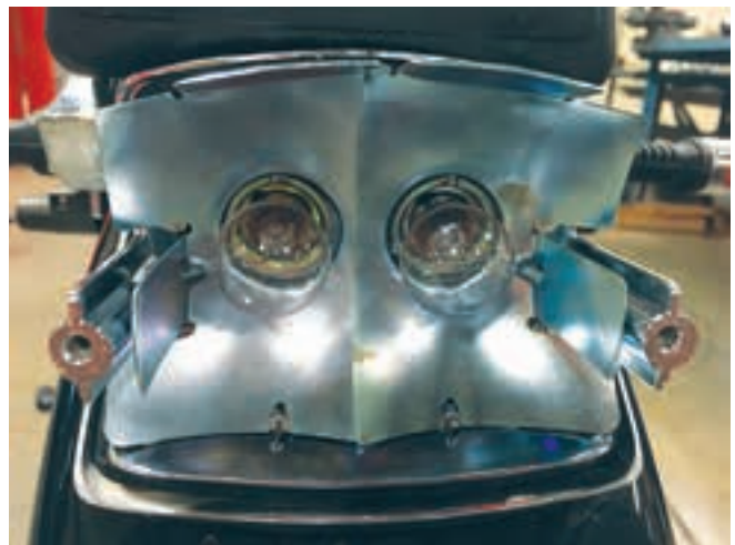
Figure 12-13. Taillight and brake light brightness is often increased by using two bulbs in a single light housing.
