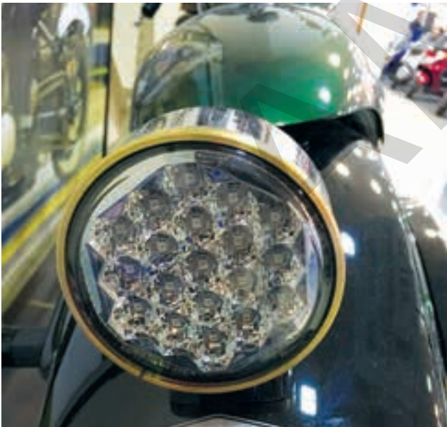
Figure 12-11. LED taillights are brighter and more durable than incandescent bulbs.
