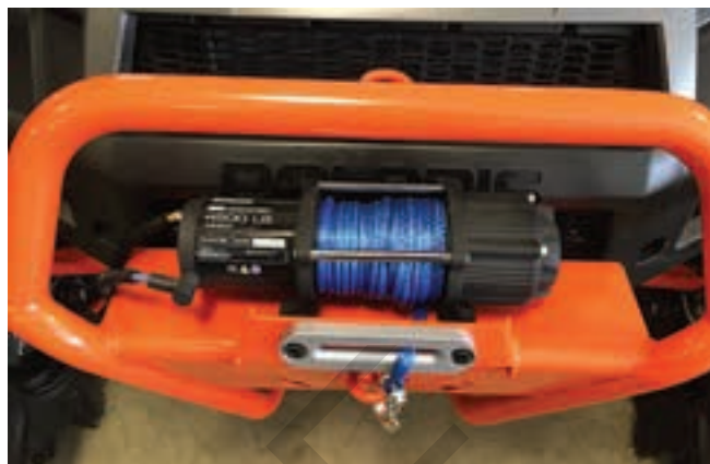
Figure 12-35. Winches on ATVs and UTVs are helpful if the vehicle gets stuck or needs to be loaded onto a trailer.
