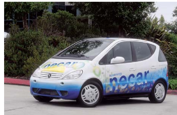
Figure 5-20. Cars operating on hydrogen fuel cells have moved beyond the experimental phase and are being operated in small numbers in Germany, Japan, Singapore, and the United States. This is a demonstration vehicle based on a Mercedes-Benz automobile model. (DaimlerChrysler)
