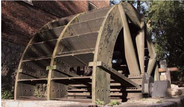
Figure 5-9. For thousands of years, waterwheels have been used to harness the energy of flowing water. This large wheel is part of a restored gristmill located alongside a creek. The wheel is more than 10' in diameter.
